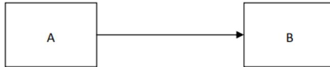
FIGURE 38 – Mode de transmission simplex.
